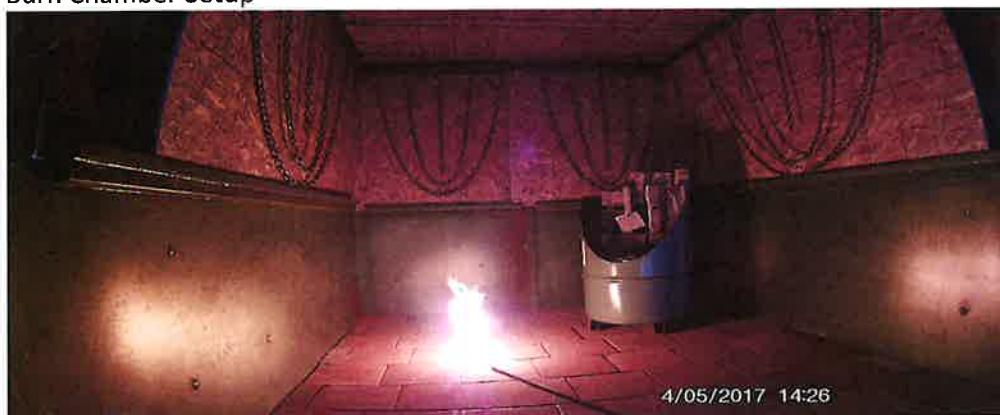
(c) Burn Chamber Setup
